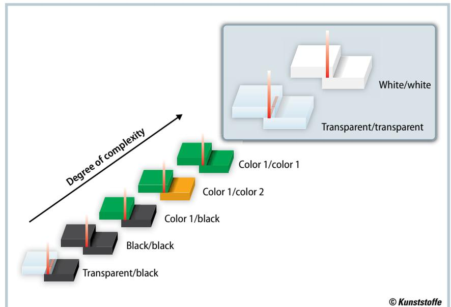
**Fig. 4.** The absorber effect makes combinations of transparent and black components easy to join with laser transmission welding, whereas the pair white/white is the most difficult (figure: Treffert)
