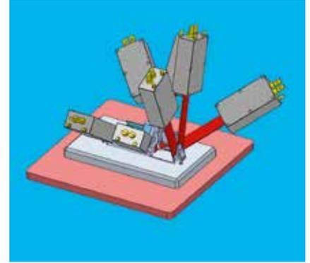
**Fig. 3.** Modularly constructed line arrays are possible with four or seven laser modules (figures: Limo)
