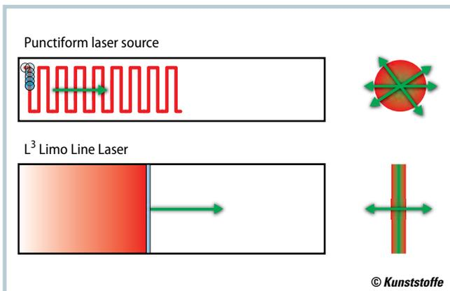
**Fig. 1.** Unlike point-shaped lasers, which have a round beam profile, line lasers process the entire surface simultaneously and uniformly (figure: Limo)
