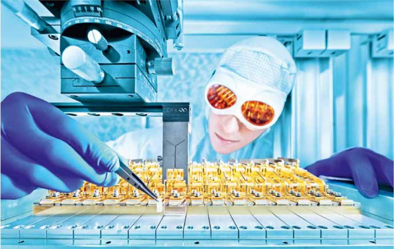
Because the laser line is separated into 15 individually controlled line segments with an area of 1.5 mm by 21 mm, the laser beam strikes only the specifically desired welding points on the plastic parts (figure: Limo/Markus-Steur.de)
